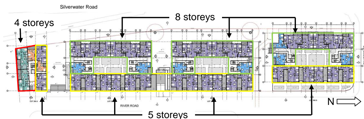
Figure 12: Plan configuration of the buildings at Lot 306 indicating number of storeys
